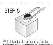
With inked side up apply flux to bottom of redi-prong by holding it in tweezers and dabbing rediprong in thin layer of flux on bench block.
